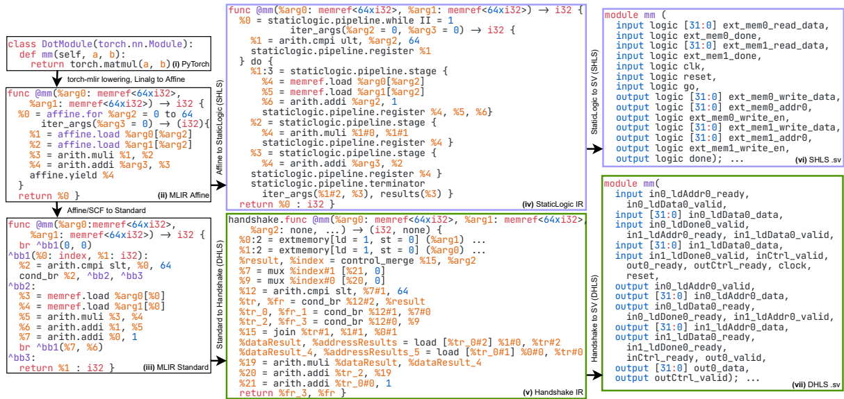
Figure 2: A PyTorch example (i). The input IRs for two backend flows as affine loops (ii) and a CFG (iii). The mid-level IRs for each flow as a static pipeline (iv) and a dataflow graph (v). SystemVerilog modules generated by each flow (vi) and (vii).
