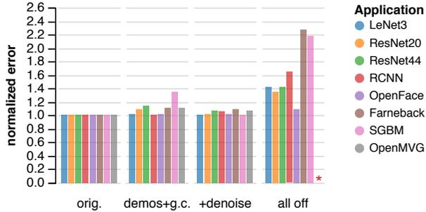
Figure 4: Each algorithm’s vision error, normalized to the original error on plain images, for two minimal ISP pipelines. The *demos+g.c.* pipeline only enables demosaicing and gamma compression; the *+denoise* bars also add denoising. The *all off* column shows a configuration with all stages disabled for reference.
